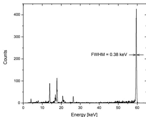
Figure 1: <sup>241</sup>Am spectrum of HPGe-detector.
