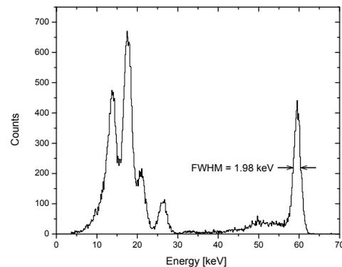
Figure 2: <sup>241</sup>Am spectrum of Si(Li)-detector.
