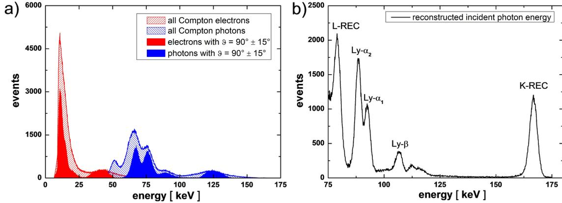
**Figure 3.** Reconstruction of the Compton events inside the detector: a) By applying several conditions the true Compton events, consisting of the recoil electron and the scattered photon, were identified. A further selection with respect to the polar scattering angle  $\vartheta$  takes into account only the Compton events with the maximum polarization sensitivity. b) Energy spectrum of the reconstructed Compton events, given by the sum energy of the recoil electron and the scattered photon.
