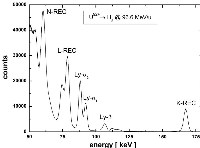
**Figure 2.** Energy spectrum of x-rays arising in the collision of  $U^{92+}$  with  $H_2$ , recorded at a beam energy of 96.6 MeV/u. To exclude contributions by Compton scattering and double hits inside the detector, only events with exactly one inelastic interaction were taken into account.
