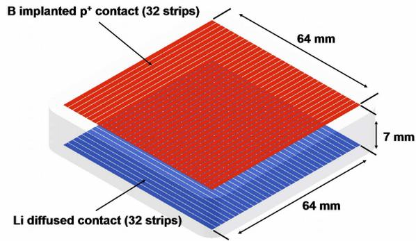
**Figure 1.** Left: Photograph of the Si(Li) Compton polarimeter developed within the SPARC Collaboration. The crystal and the preamplifiers are located in the head of the detector which is connected to a LN2 dewar. Right: Sketch of the detector crystal with the front side and the back side each being segmented into 32 strips giving a structure of 1024 pseudo-pixels.
