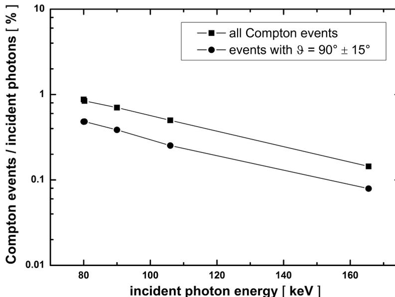
**Figure 5.** Experimental data for the polarimeter efficiency of the Si(Li) detector. About 50 % of the reconstructed Compton events show polar scattering angles  $\vartheta$  near  $90^\circ$  providing the maximum polarization sensitivity.
