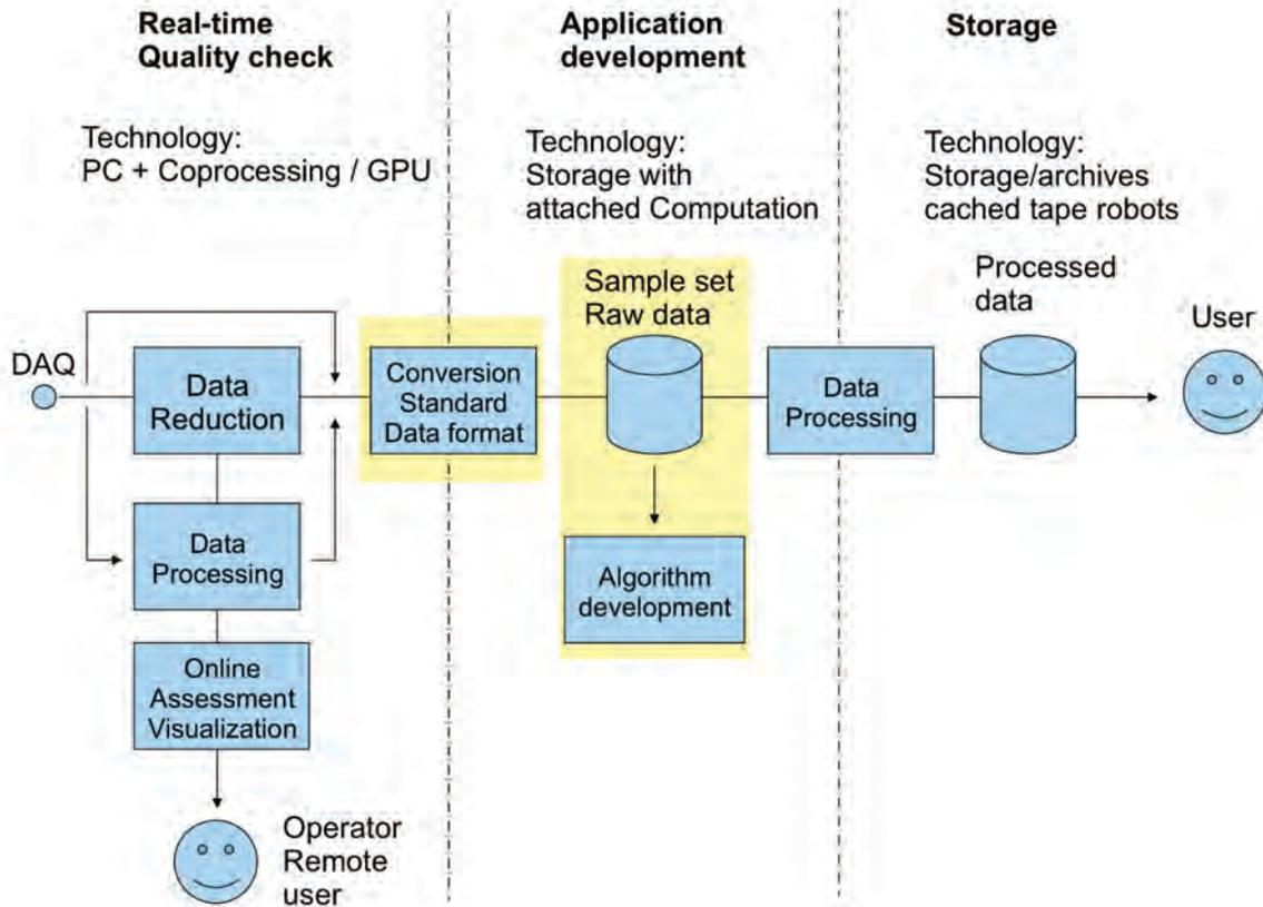
Figure 1: Simplified scheme of data flow at PNI facilities.
