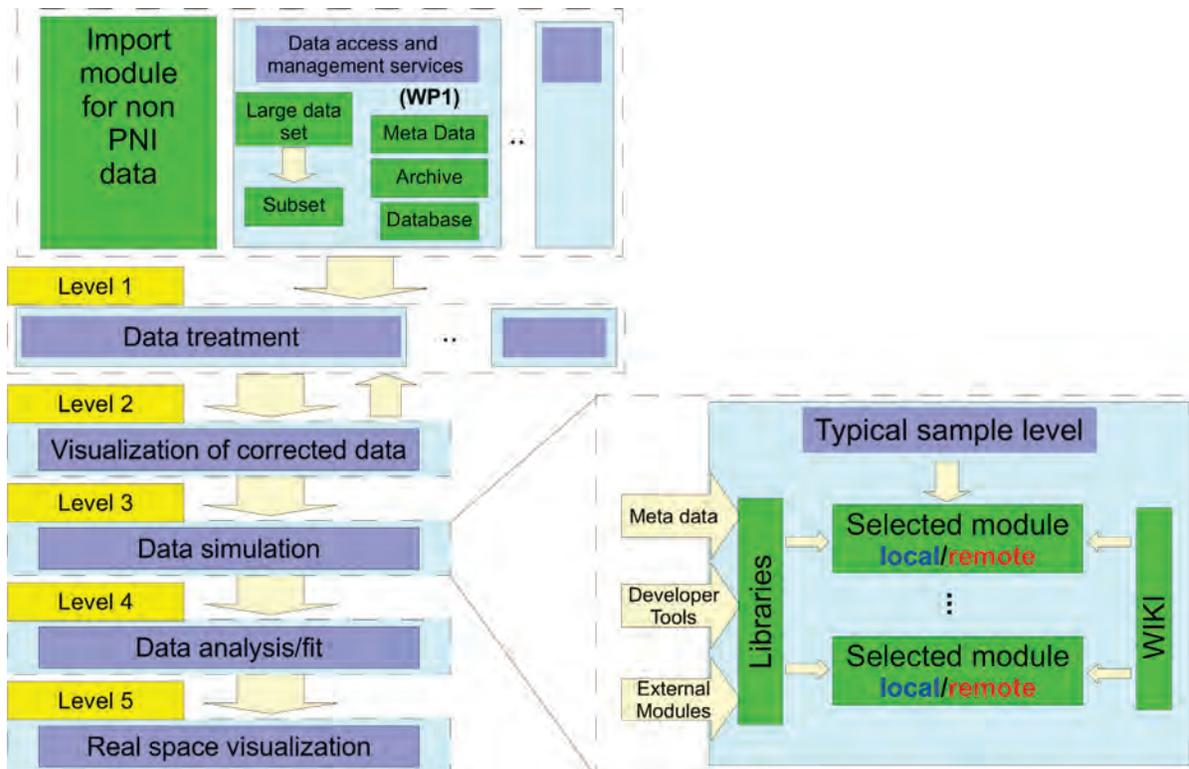
Figure 2: Schematic interdependency of the key components and the work flow of the planned data correction, analysis and visualization framework.
